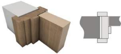
FRAME TYPE ONE - LINING AND STOP
