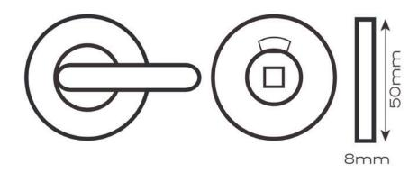
19027K 50x8mm large turn & key operated emergency release/indicator
